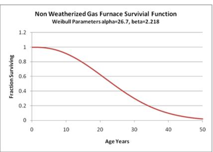
**Figure 65: Weibull Distribution for Non-weatherized Gas Furnaces** Source: GTI analysis of data from TSD Chapter 8<sup>10</sup>
